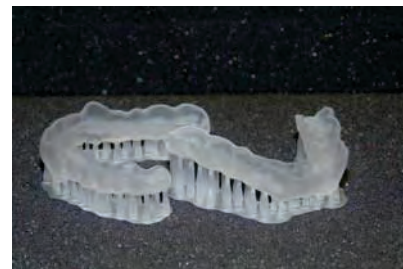
The splints after light curing and before separation of the support.
