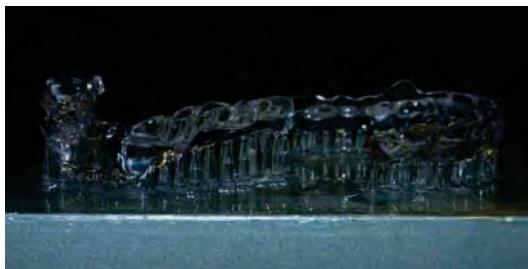
Immediately after the printing process in the ASIGA-Pro2. The splints here are still on the build platform.
