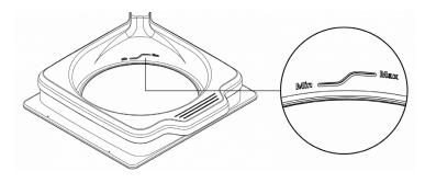
If there is leftover resin in the tank from the previous print, use the provided resin wiper to stir the resin before printing. This ensures that the resin is properly mixed and clean.
